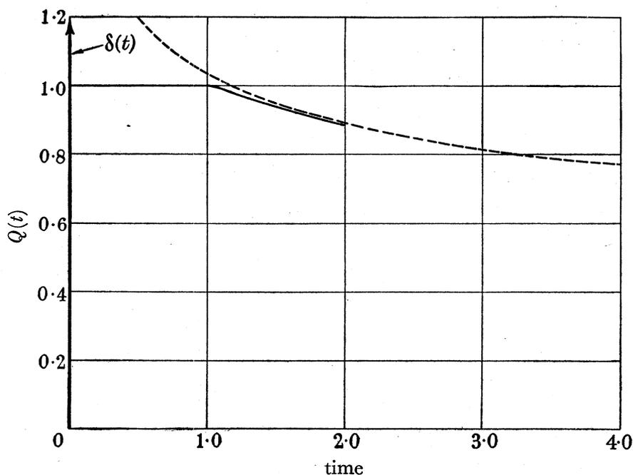
FIGURE 7. Variation of  $Q(t)$  with time according to exact (—) and asymptotic (---) solutions.
